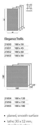
chamfered edges,gap size: 50 x 50 mm
